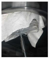
Place a cloth soaked in a foamy soap solution over the brush and clean the suction pipe. Intense soiling should subsequently only be cleaned with the brush. Then dry the damp suction pipe with a cleaning cloth over the head of the special brush.
